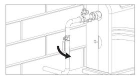
1. Turn off the water supply by turning off the valve. Drain the pipes by turning a tap on inside the home that is fed water via the filtration system to reduce the systems' water pressure.
