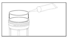
5. Lubricate the O-ring with clean silicone grease. Do not use petroleum jelly. Insert O-ring into the groove. This step is important to ensure a proper filter housing seal. Make certain the O-ring is seated level in the groove.
