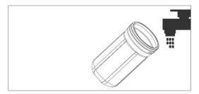
4. Discard the used filter cartridge. Wash the filter housing with dish soap and warm water using a non-abrasive sponge or cloth. Rinse thoroughly. Fill 1/3 with water, add one tablespoon of bleach and scrub to disinfect. Rinse thoroughly and dry.
