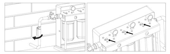
7. Turn on the water supply. Press the pressure-relief button. Check for leaks.
