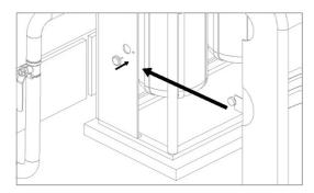
8. Assemble the cover and lock via the threaded lock screws.
