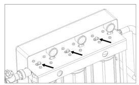
2. Remove the cover and press the red pressure-relief button.
