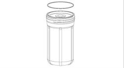
3. Using the wrench provided with the unit, unscrew the filter housing, then remove the large O-ring, wipe clean, and set aside.
